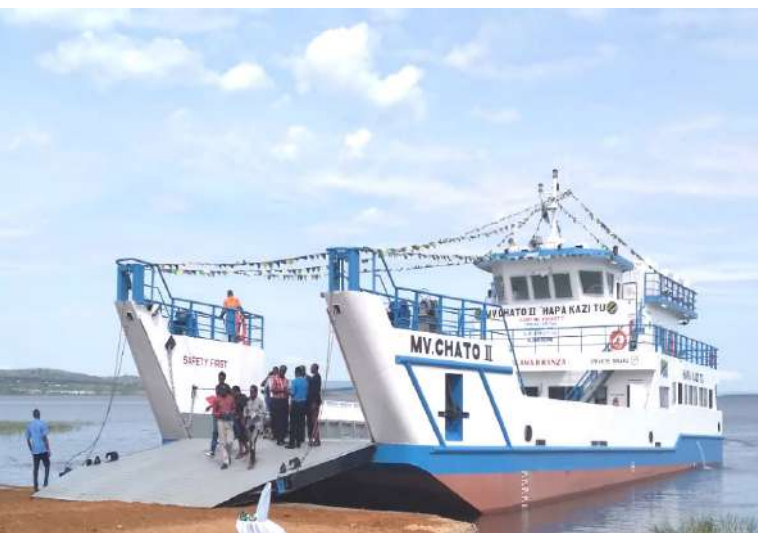
A new ferry, Mv Chato II-Hapa Kazi Tu, plying the Chato – Mharamba-Nkome routes including the neighbouring islands of Senga, Bukondo and Izumacheli in Lake Victoria, Geita Region. It has the capacity to carry 100 tons, 200 passengers and 10 vehicles.
